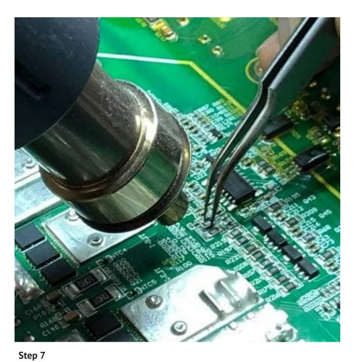
Use hot air station for add first resistor 56 Ohm.
