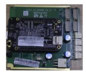
Integrated control board(A113D Control board), need to use the OTG cable (Micro usb - USB A)
