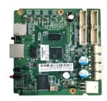
Combined control board, it's composed of IO board and BB board
